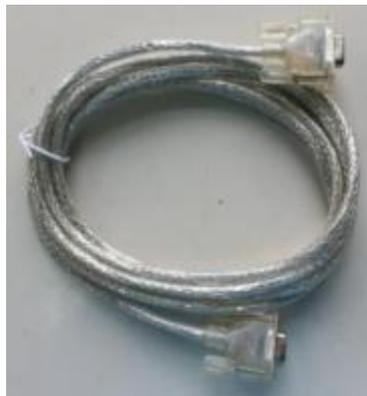
Figure 8 RS-232 serial cable
